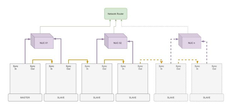
Orange Arrow is the Sync Wire / Audio Cable Purple is the Kinect Azure USB data Cable Green is the Network cables and Router
